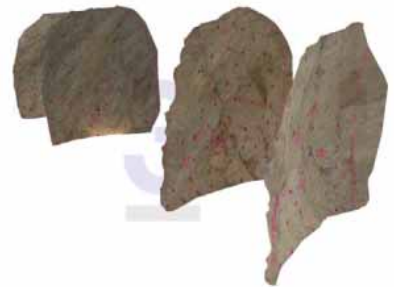
Figure 13: Subsequent 3D images of a drift tunnel excavation in an underground marble mine.
