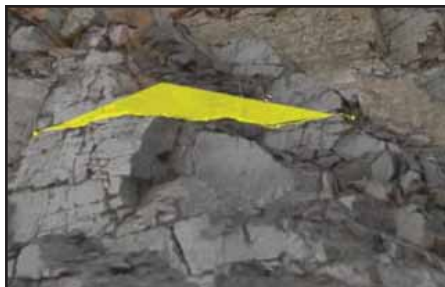
Figure 5. A discontinuity trace marked by a 3D poly-line. A plane is fitted through the sampling points. Its orientation corresponds with the orientation of the marked trace.
